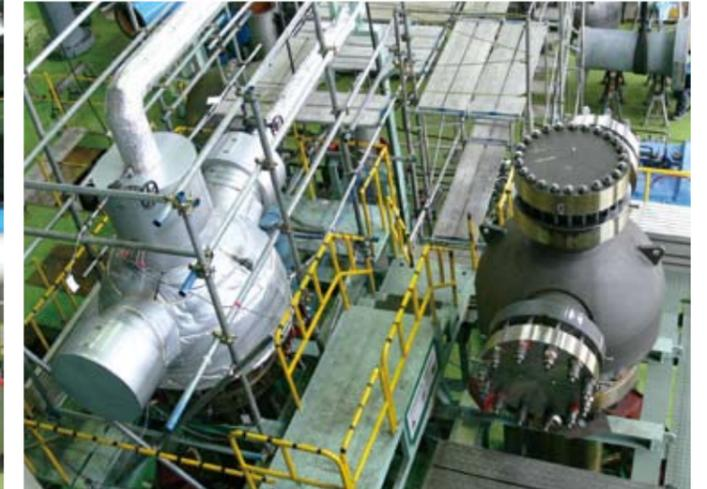
Torishima understands the need to provide a high temperature and high pressure test loop for our boiler circulation pumps.
