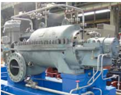
Water Transfer Pump for Salaf Pump Station (Saudi Arabia) Pump type: MHH300/4, Delivery year: 2010 Duty: 1,116m 3 /h at 615m, Power: 2,840kW
