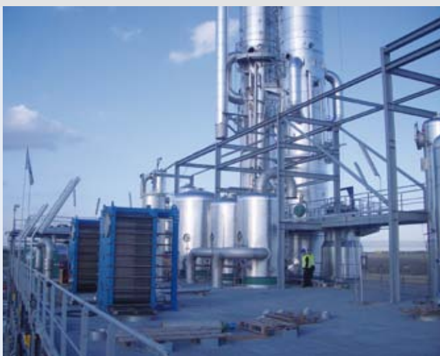
Condensation of bioethanol.
